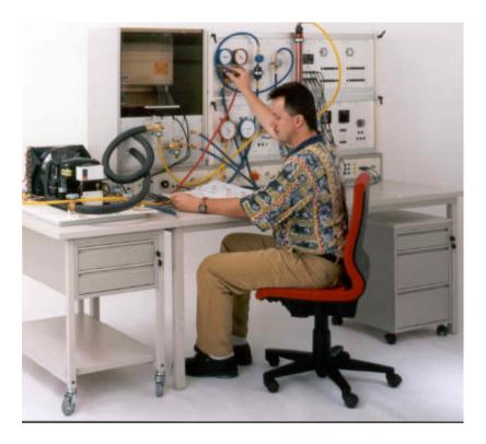
This new developed experimental station for refrigeration and air-conditioning training permits refrigeration and air-conditioning tests to be conducted in the normal cooling, air-conditioning and deep-freeze ranges, the electrical circuits to be set up, and measurements to be taken.
